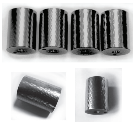
Figure 6. Textured specimens with various relative area of microgrooves F_k
