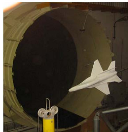
Fig 8. SHARV in Ø5m wind tunnel at the Institute of Aviation in Warsaw
