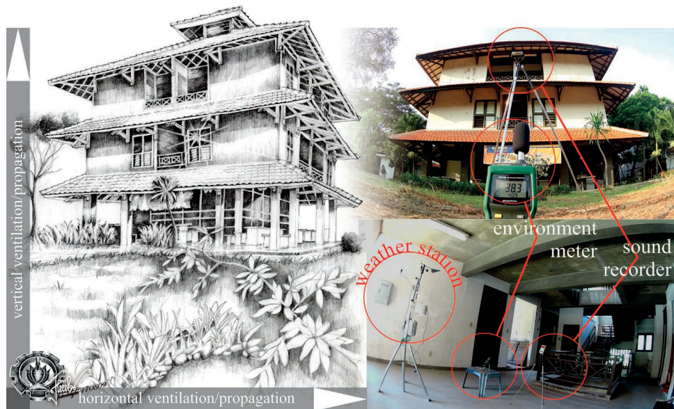
Fig. 3. Measurement method and instruments Source: Author's sketch and photograph, May-August 2017.
